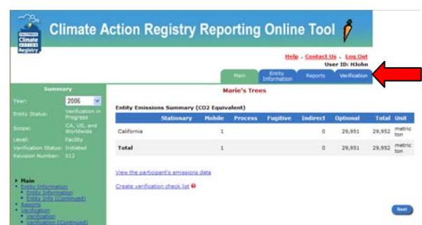
**NAVIGATIONAL TREE.** Each section of the CARROT application is listed in the green section on the left hand side of the screen. This navigational tree links to different sections. The link highlighted in **bold black** font indicates your location in CARROT.
